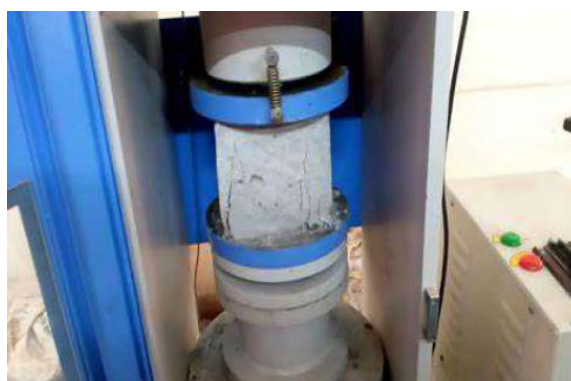
Fig. 8. Compressive strength test.
