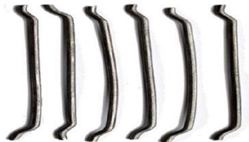
Fig. 2. Straight steel fibers with hooked ends.
