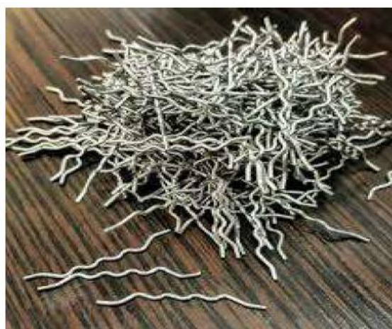
Fig. 4. Steel fibers used in the experiment.
