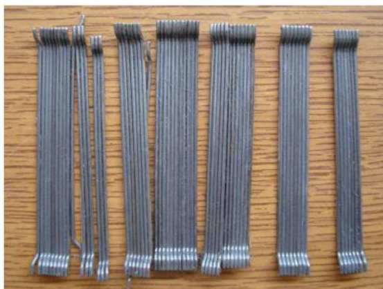
Fig. 3. Steel fibers used in the experiment.
