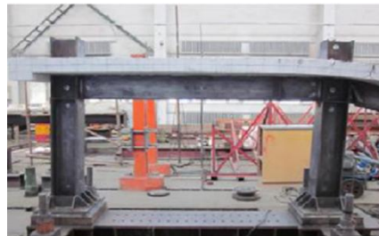
Fig. 7. Beam buckling inside connection B.
