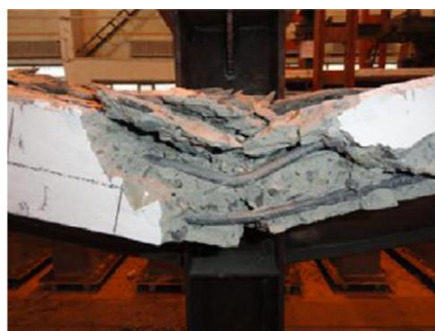
Fig. 9. Buckling of slab rebar.
