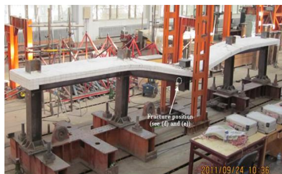
Fig. 5. General view of the tested steel frame after loading.
