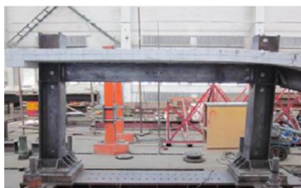
Fig. 7. Beam buckling inside connection B.
