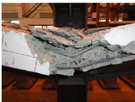
Fig. 9. Buckling of slab rebar.
