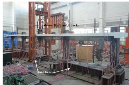
Fig. 3. The laboratory frame under investigation along with the equipment used.
