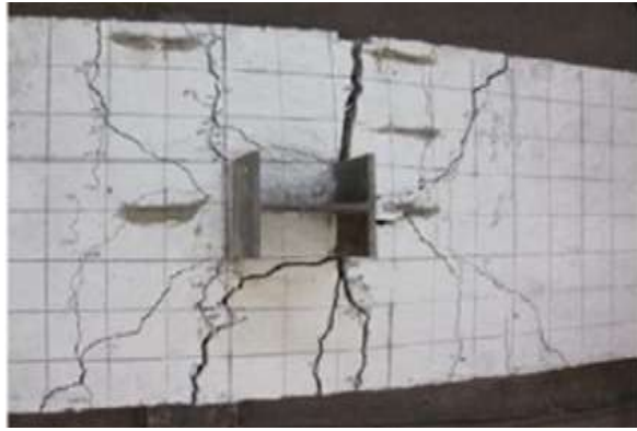
Fig. 10. Cracks in the slab at connection area B.
