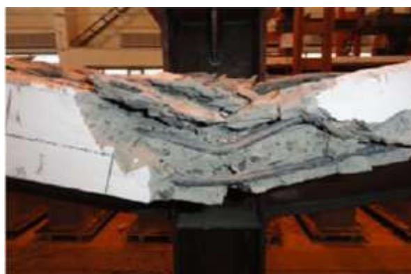
Fig. 9. Buckling of slab rebars.
