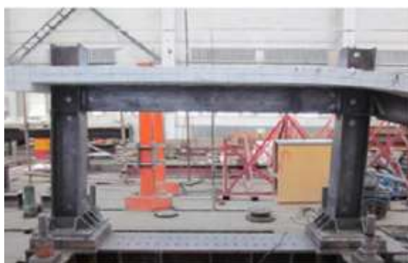
Fig. 7. Beam buckling inside connection B.
