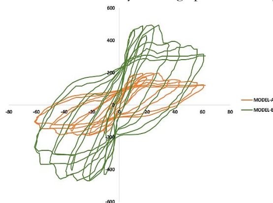
Fig. 16. Hysteresis diagram of model A, B under cyclic loading.
