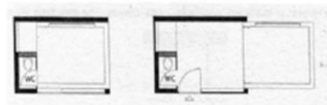
Expandability through sliding relocation of the prefabricated model Fred, Austria, Study, 1999 Architect: Oscar Leo, Johannes Kaufmann Contracted and expanded module
