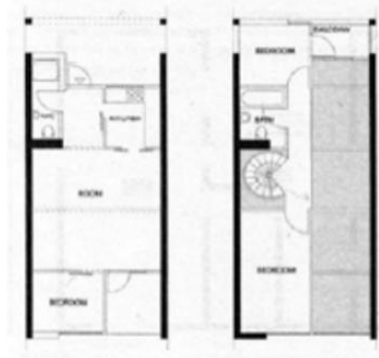
Vertical expansion in a given space, growth capability with high ceiling height allocation and general separation capability Projekt Wohnhaus, Germany, Study, 1984 Architect: Anton Schweighofer First & Second possible Floor Plan
