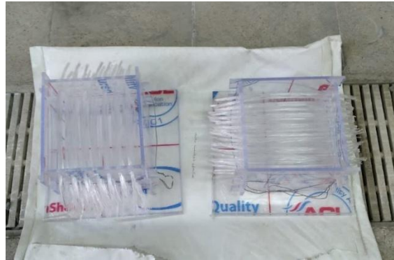
Fig. 3. Two molds with optical fibers.
