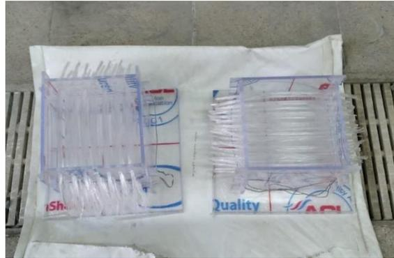
**Fig. 3.** Two molds with optical fibers.
