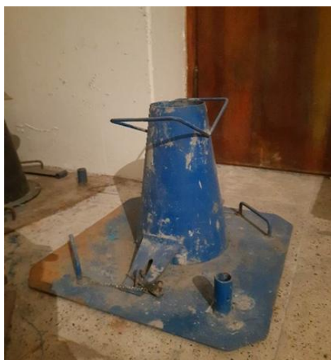
Fig. 6. Slump test mold.
