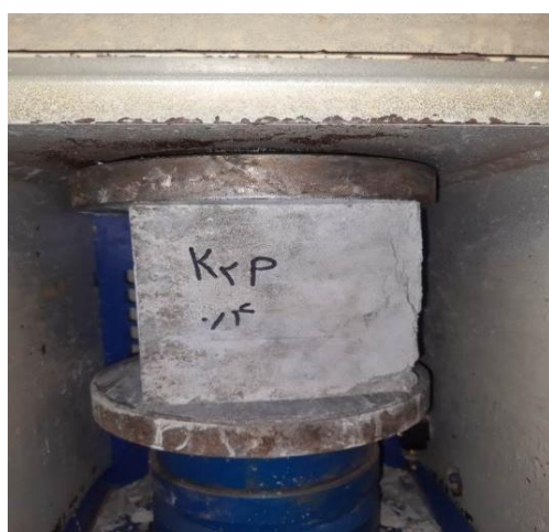
Fig. 11. 28-day concrete sample with 0.4% fibers.
