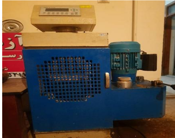
Fig. 5. Concrete compressive strength determination device.
