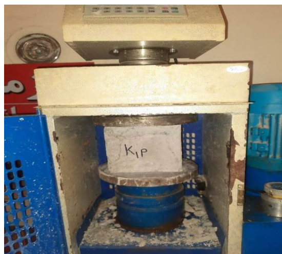
Fig. 9. 28-day sample with 0.2% rock wool fibers.
