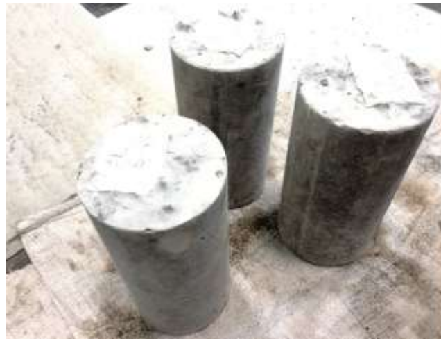
Fig. 4. Cylindrical samples for testing tensile strength.
