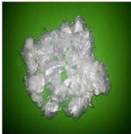
Fig. 1. Polypropylene fibers after separation by hand.
