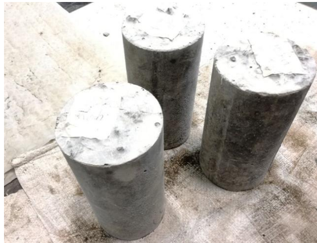
Fig. 4. Cylindrical samples for testing tensile strength.
