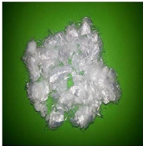
Fig. 1. Polypropylene fibers after separation by hand.
