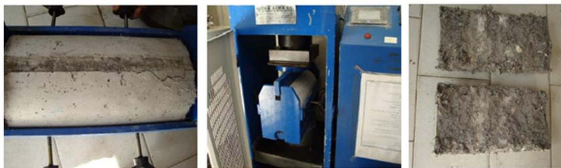
Fig. 5. Testing to determine the tensile strength of cylindrical specimens using the Brazilian method.
