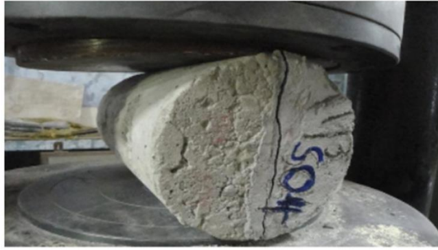
Fig. 2. Image of the concrete sample in the testing machine.
