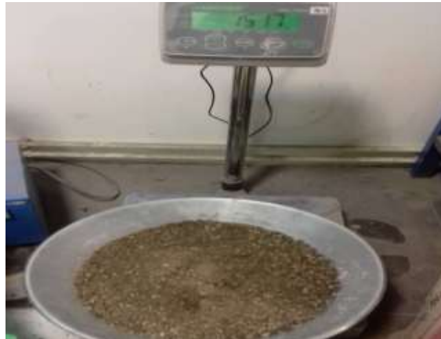
Fig. 7. Weighing of dry materials.
