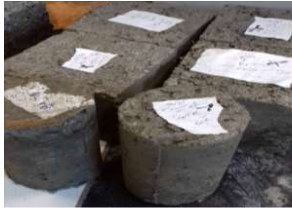
Fig. 9. Concrete samples after removing from the molds.
