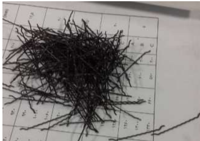
Fig. 4. Sinusoidal metal fibers with two hook ends with a diameter of 0.8 mm.
