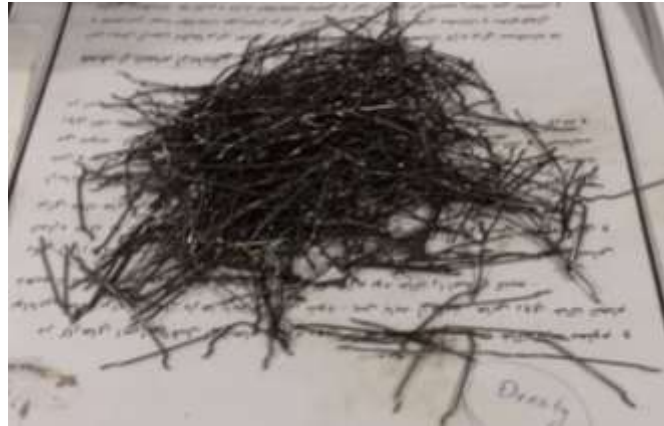
Fig. 3. Metal fibers with two hook ends with a diameter of 0.5 mm.
