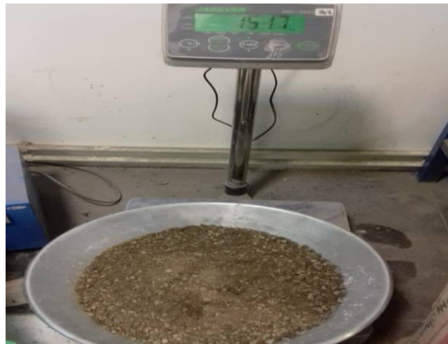
Fig. 7. Weighing of dry materials.
