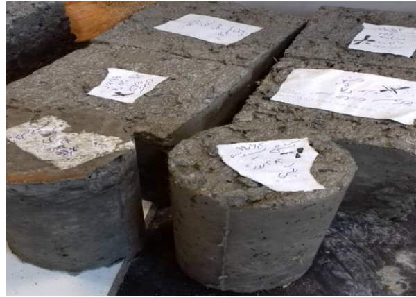
Fig. 9. Concrete samples after removing from the molds.
