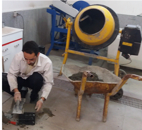
Fig. 2. The process of concrete production: mixing and pouring.
