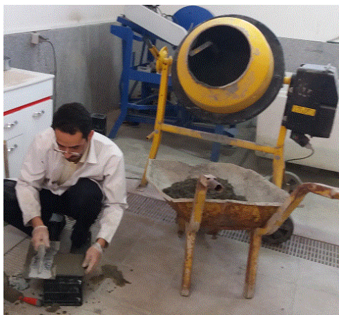
Fig. 2. The process of concrete production: mixing and pouring.
