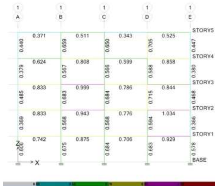
Fig. 8. The stress percentage in the designed sections of Model 1 in ETABS software.
