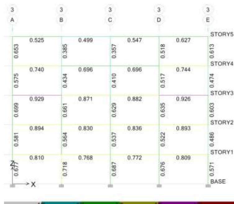
Fig. 6. The stress percentage in the designed sections of Model 1 in ETABS software.
