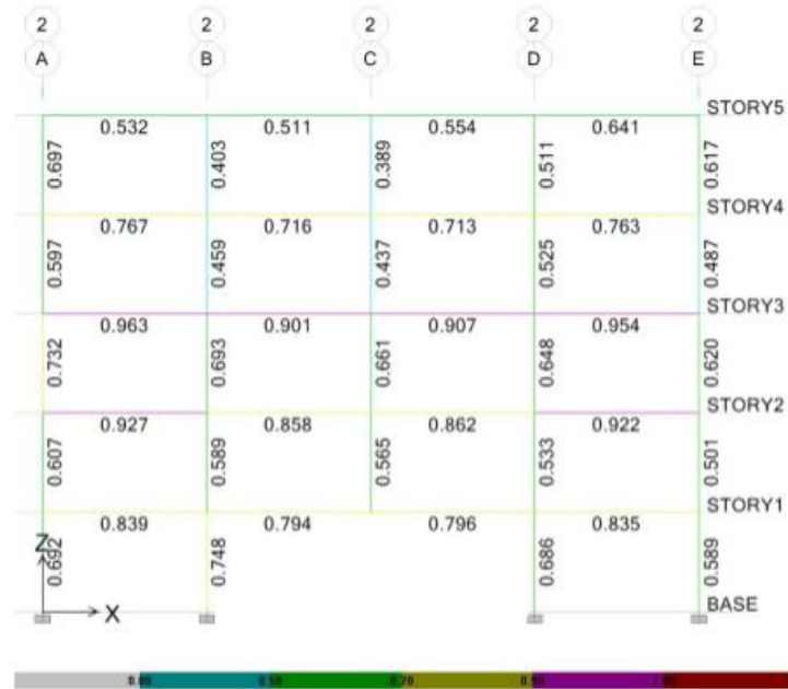
Fig. 7. The percentage of stress in the designed sections of Model 1 in ETABS software and with progressive failure.
