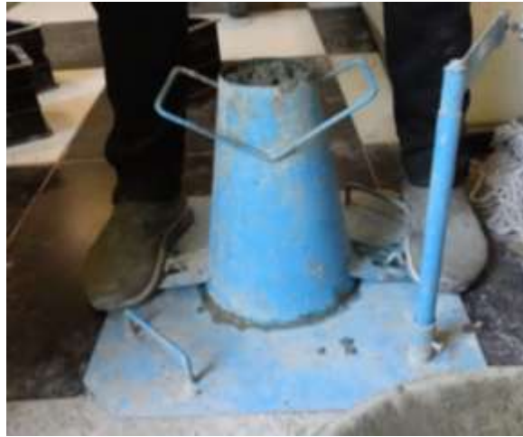
Fig. 9. Poured concrete in the slump cone.
