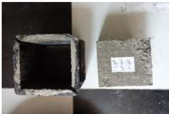
Fig. 8. Concrete samples 24 hours after construction.
