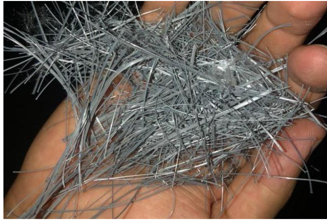
Fig. 3. Needle-shaped polyolefin fibers.
