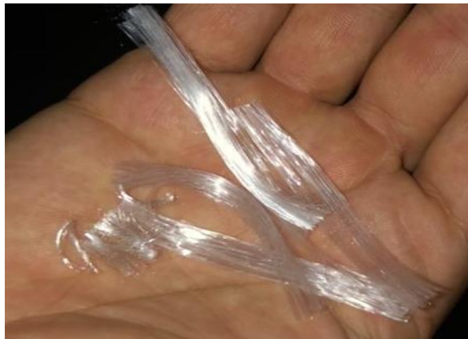
Fig. 4. Polyolefin network fibers.
