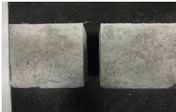
Fig. 12. Cracking pattern of concrete samples after pressure test.
